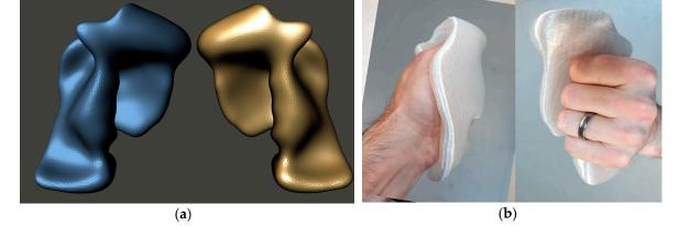
**Figure 6.** Latest design solution: (**a**) final CAD models of the pair of customised wheelchair racing gloves; (**b**) the 3D printed gloves being tested for fit using Premium PLA (Raise3D) material.
